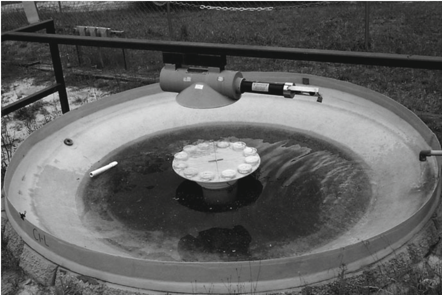
Fig. 19.3 Special containers housed fish eggs and were exposed under known geometries with doses measured by TLDs. The photo depicts one of several egg exposure arrangements that were tested
