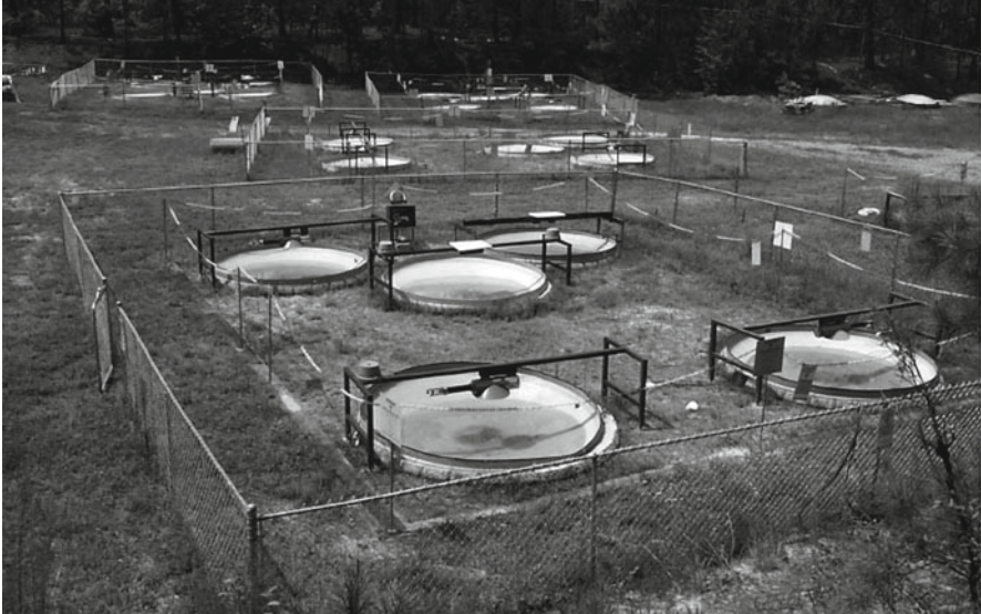
Fig. 19.2 Photo of a portion of the LoDIF facility, showing a pad with five mesocosms, three of which have sealed Cs-137 sources above them (cylinders mounted on frames that cross the mesocosm). Eight replicate pads exist within the LoDIF, resulting in 40 mesocosms
