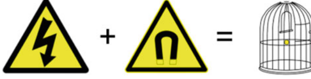
Fig. 2.1 Cartoon of a Penning trap being a cage for a charged particle by a combination of electric and magnetic fields
