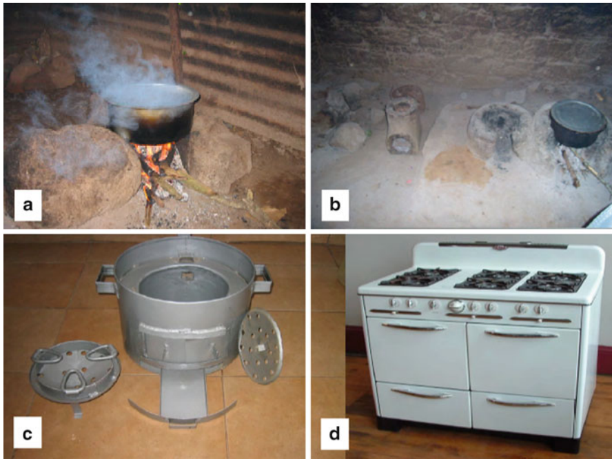
Fig. 16.3 Typical stoves include (a) 3-stone stove suitable for any type of biomass, (b) improved stoves made from clay most commonly used with fuelwood, (c) metal improved stoves that can accommodate both biomass and charcoal, and (d) modern stoves that use LPG
