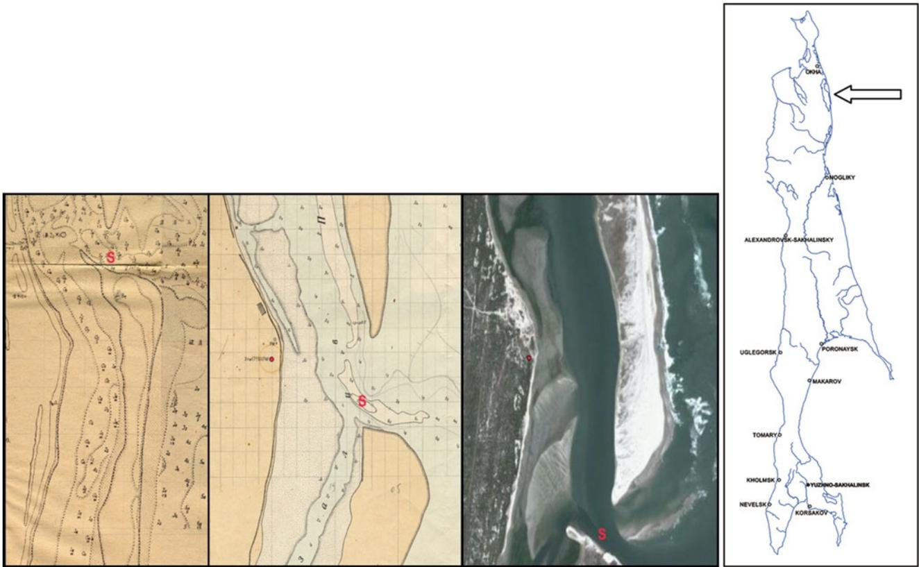
**Fig. 3.10** Shift of the Piltoon Strait to the south, determined by navigational maps, dated 1920 and 1972, and (space image) 2006 (S – the greatest depths in fairway)
