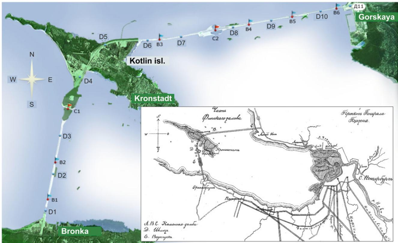
**Fig. 7.13** Modern plan of the St. Petersburg Flood Protection Facility (C1, C2 – gates for vessels; B1–B6 – water gates; D1–D11 – dams) and first project of protection contracture by Federic Basen (1824–1827)
