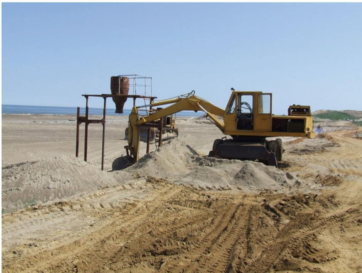
**Fig. 3.15** Sand extraction at the Keutu Lagoon
