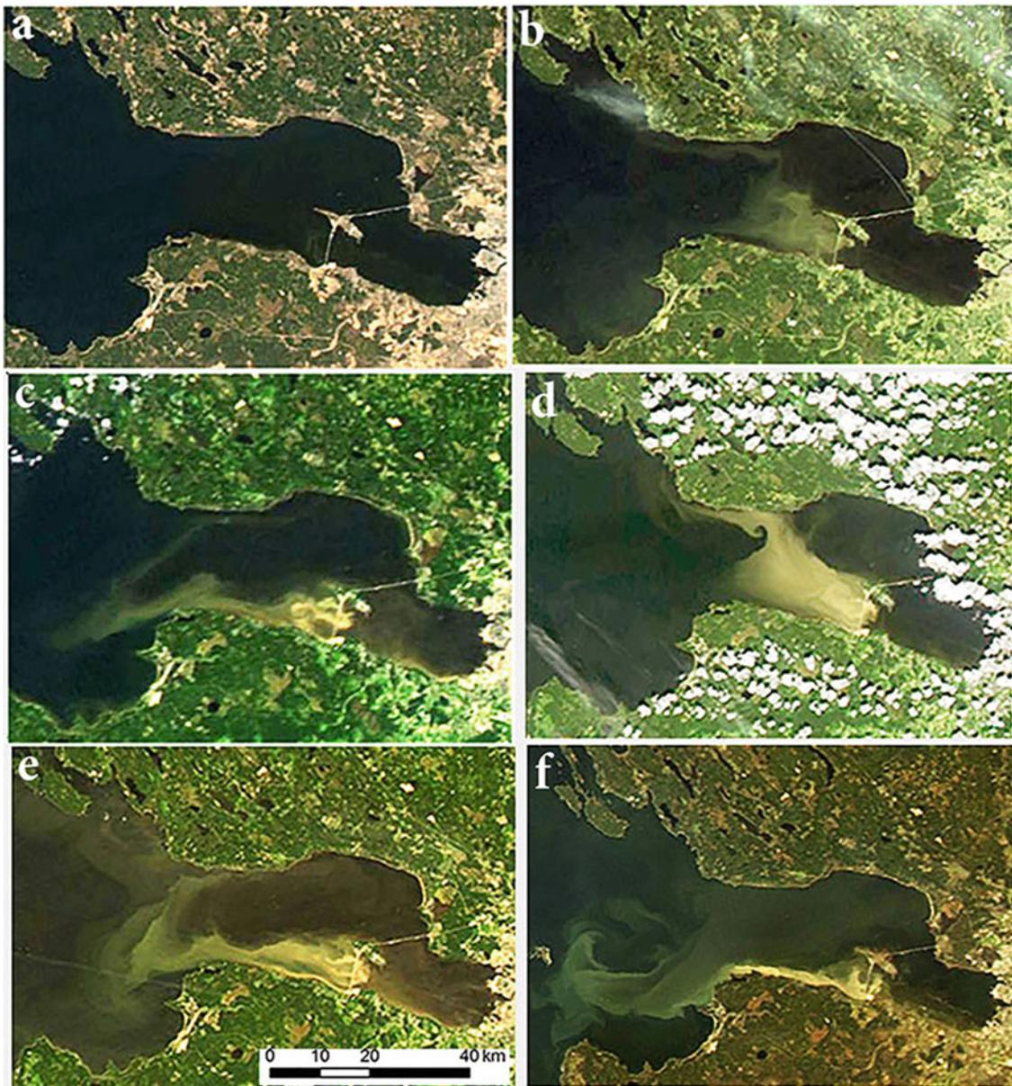
**Fig. 7.14** Satellite images obtained from sensor MODIS: (a) image from April 20, 2014, the usual view of the aquatic system before hydro-technical work has started; (b) from May 17, 2014, hydro-technical works, already started, can be observed in the stratification of water masses and the presence of upwelling; (c) image from June 15, 2014, presence of hydro-technical works, winds of northeastern direction, decreasing of the sea level; (d) from July 7, 2014, intensification of
