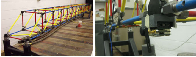
Fig. 6 Truss structure and an installed Imote2 sensor node
