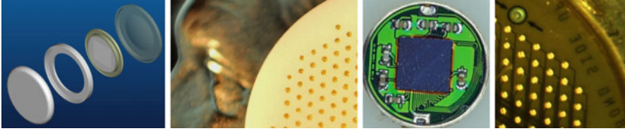
Fig. 7.7 Hermetic case assembly. From left to right : An exploded view of the case, showing titanium case pieces, feedthrough, and polyurethane header. A view of the feedthrough on a US nickel 5-cent coin. Circuit board and chip soldered into the case. Electrode array bonded to the outside of the feedthrough
