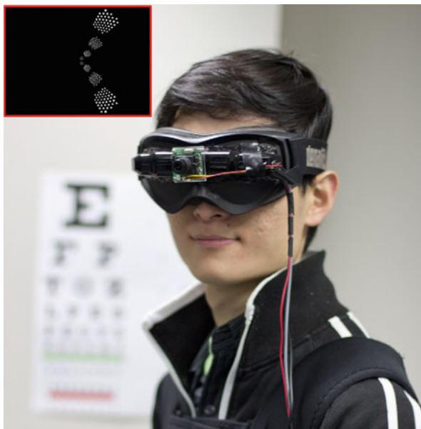
Fig. 17.5 Real-time head mounted simulator for Gennaris showing 8 implant tiles mapping into the user's visual field. Note the top left insert shows what the user sees with all electrodes activated
