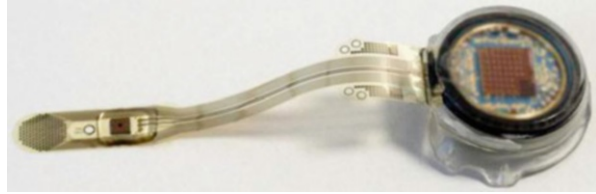
Fig. 8.4 IRIS™ Implant showing the Application Specific Integrated Circuit (ASIC) part in its circular case and the polymer foil with the electrode array at its extremity
