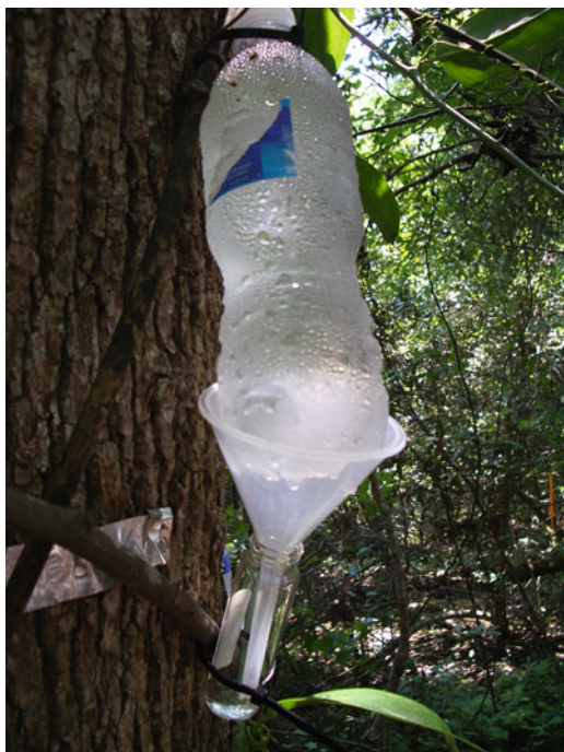
Fig. 13.20 Simple apparatus developed by the author to collect tritiated water vapor from the riparian forest growing above tritium-contaminated groundwater. See Vroblesky et al. (2009) for more information (Photograph by author).
