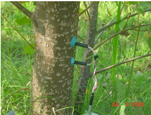
Fig. 9.2 A thermocouple dissipation probe (TDP) installed in the trunk of a poplar tree at a phytoremediation site near Elizabeth City, NC (Photograph by author).
