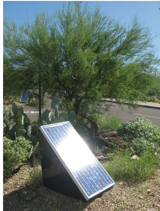
Fig. 3.19 A leaf and a solar panel essentially perform the same task; harnessing the sun's energy for storage in a more useable form. Here, the solar panel provides power to a battery that runs lights for a parking lot at night. The tree, a palo verde ( Cercidium microphyllum ) near Tucson, Arizona, uses the sun to generate ATP to support life (Photograph by author).
