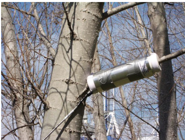
Fig. 13.4 Measurement of sap flow in a 7-year old hybrid poplar tree using the heat-balance method (Photograph by author).
