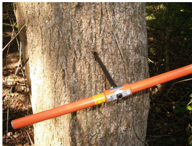
Fig. 15.1 An increment borer used to collect tree cores. The borer has been advanced but the inner sleeve not yet inserted (Photograph by author).
