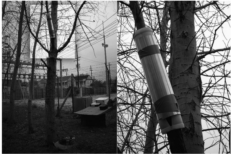
Fig. 9.1 A sap-flow heater installed on the branch of a dormant poplar tree at a phytoremediation site near Charleston, SC. The sap flow is measured along with changes in groundwater level, in a shallow monitoring well located at the base of the tree (Photograph by author).
