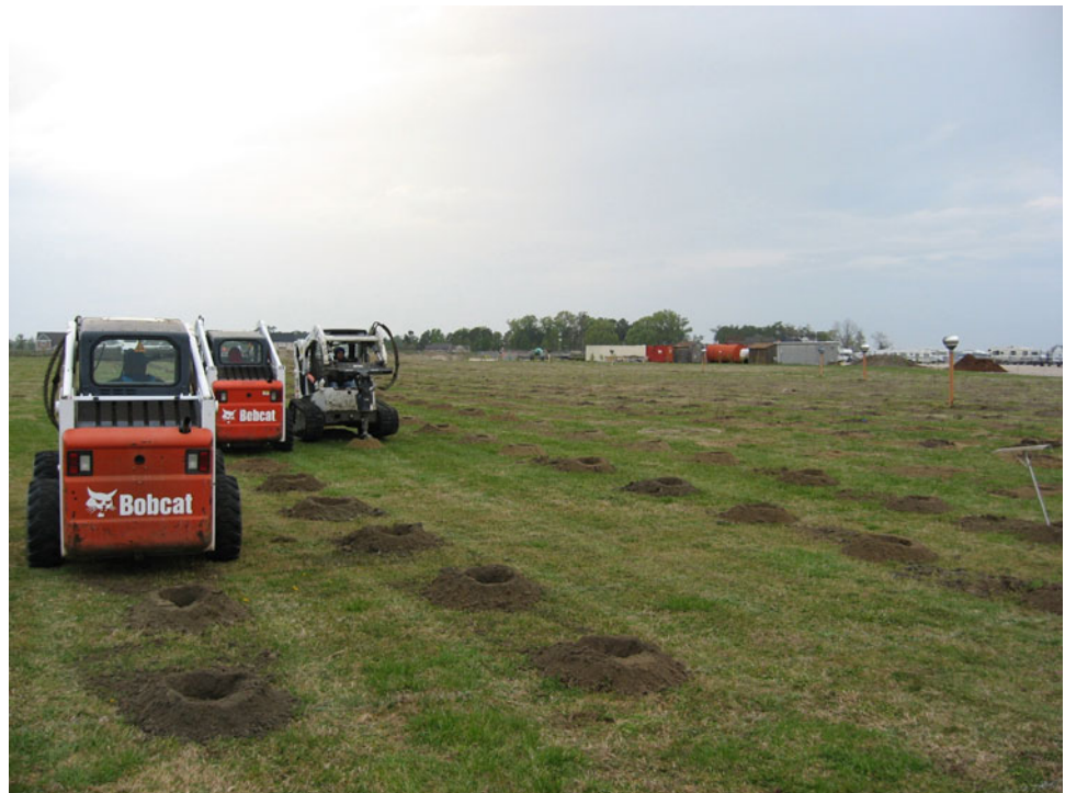
Fig. 7.4 Drilling boreholes using rotary augers prior to planting hybrid poplar cuttings, Elizabeth City, NC, United States Coast Guard Support Center (Photograph by author; see Cook et al. 2010 for further explanation).
