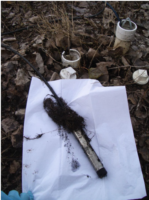
Fig. 13.14 Oak-tree roots on a water-level pressure transducer removed from a monitoring well at a phytoremediation site near Beaufort, South Carolina. These roots had not grown within the well casing and down to the water table; rather, the roots had grown in the unsaturated zone and entered the well through the well screen (Photograph by author).
