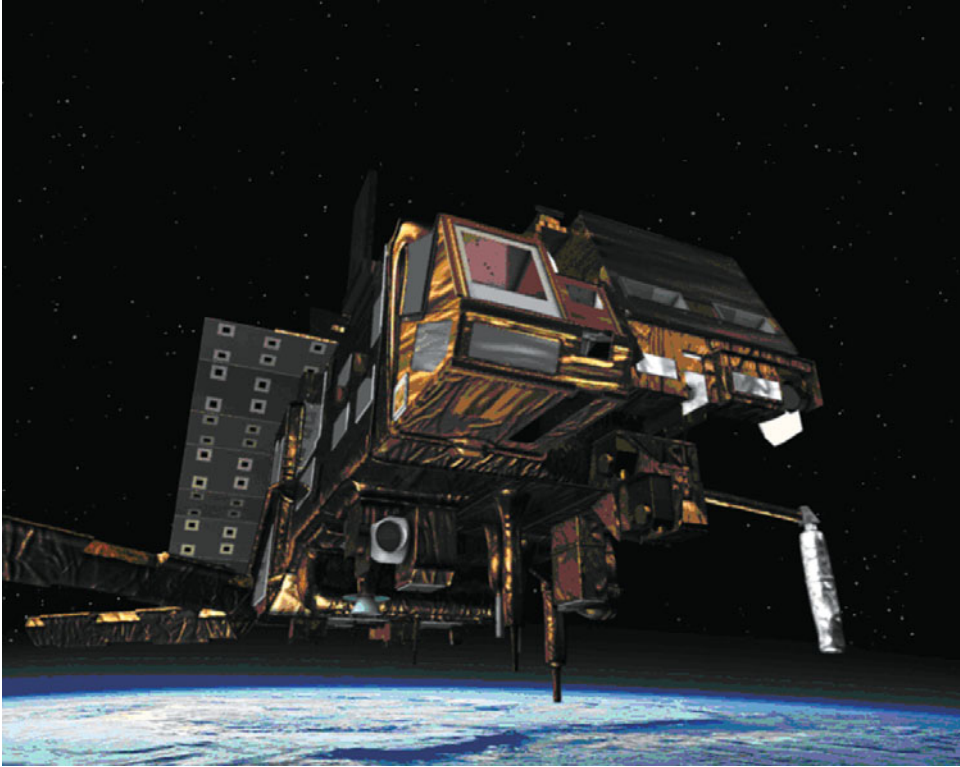
Figure 2.11. The MetOp satellite carrying the IASI instrument (European Space Agency).
