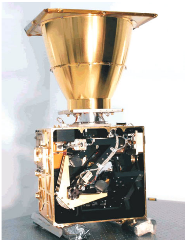
Figure 2.8. The ACE-FTS instrument (interferometer side) ( http://www.ace.uwaterloo.ca/instruments_acefts.html ).
