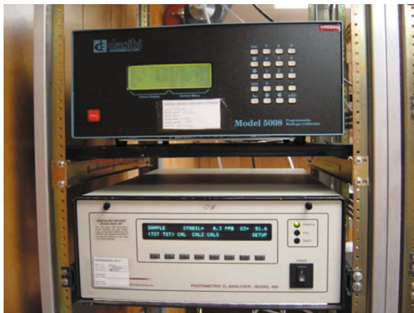
Figure 1.30. Advanced Pollution Instruments (API) Model 400E Ultraviolet Absorption Ozone analyzer (source: http://www.anr.state.vt.us/air/monitoring/htm/InstrumentInfo.htm#ozone ).
