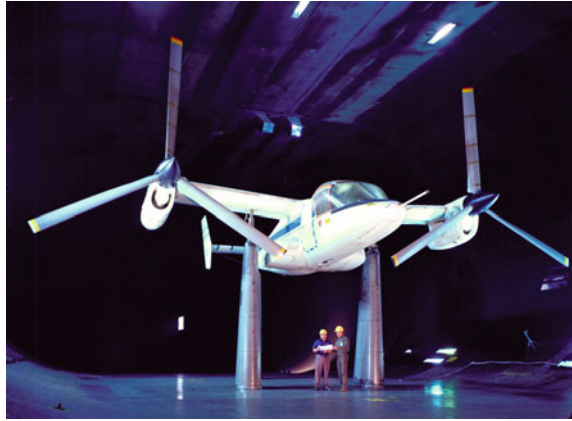
Fig. 5.1 Bell XV-15 tiltrotor research aircraft in NASA Ames 40 \times 80 ft wind tunnel (Source http://www.nasa.gov/centers/ames/images/ )
