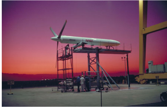
Fig. 5.17 Bell-Boeing JVX proprotor tested at NASA Ames Outdoor Aerodynamic Research Facility (OARF) (Source http://www.nasa.gov/centers/ames/images/ )
