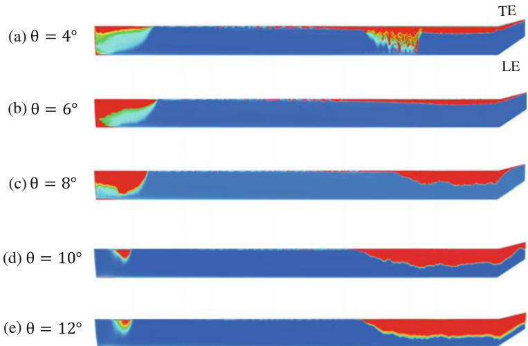
Fig. 5.52 Intermittency distributions on the S-76 lower surface ( blue laminar, red turbulent )
