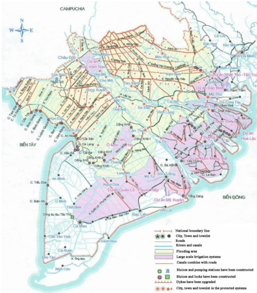
Fig. 3.16 Large scale surface irrigation systems developed in the Mekong Delta during the period of 1995–2010 (Tri et al. 2005)
