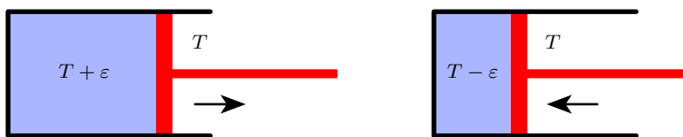
Fig. 3.14 A reversible process. Left: When the cylinder gas is infinitesimally warmer than the outside atmosphere (by \epsilon > 0 ), it expands against the piston (assumed frictionless) to do work quasi-statically on the atmosphere. Right: When the cylinder gas is made infinitesimally cooler than the atmosphere, the atmosphere pushes against the piston to do quasi-static work on the cylinder gas
