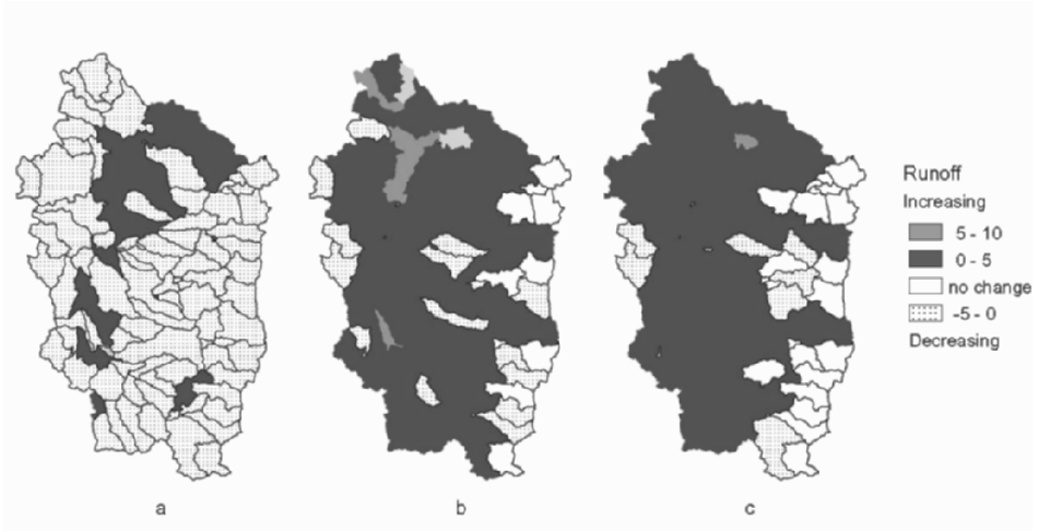
Figure 9. Percent change in surface runoff for future scenarios. (a) Conservation, (b) Development, (c) Plan Trend.
