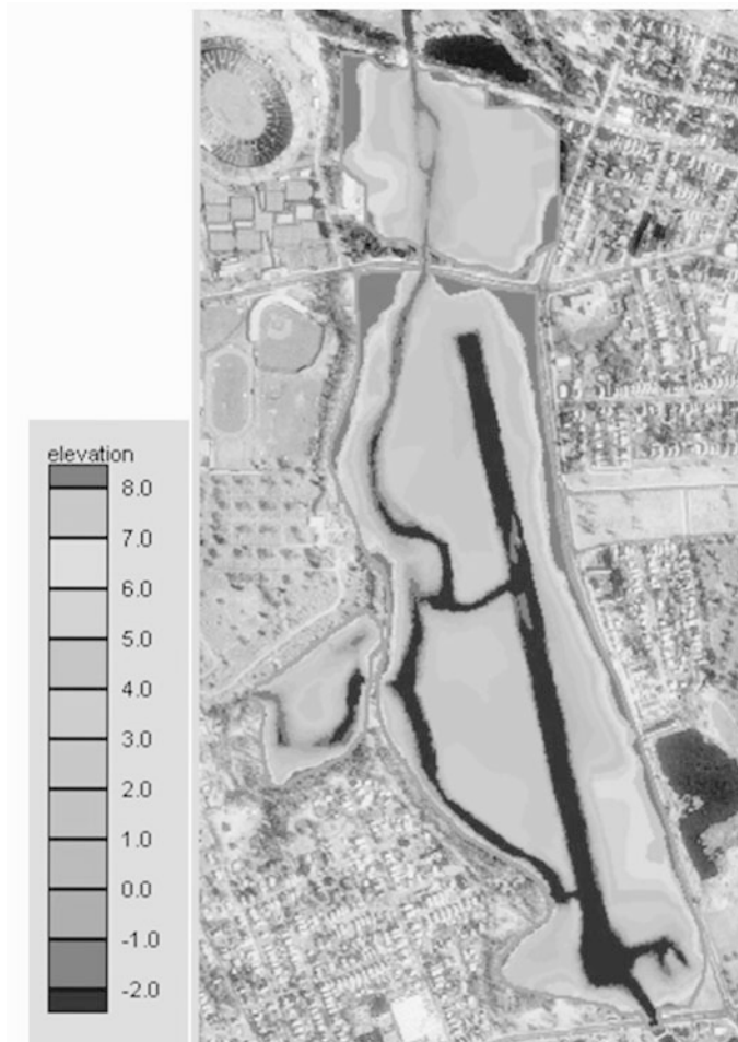
FIGURE 2.3. Two-dimensional model solution with flood limits for the West River, New Haven, Connecticut.
