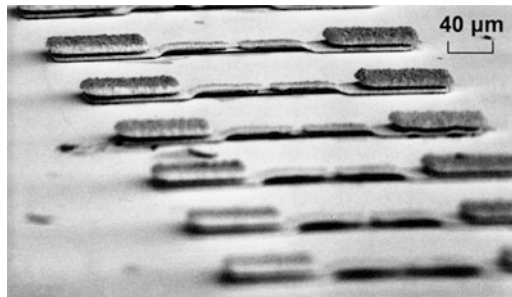
Fig. 2.6 SEM picture of two fabricated devices connected in planar approach
