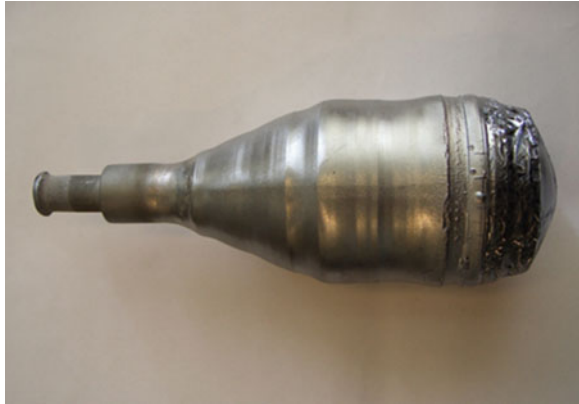
Fig. 29.2 3' diameter ingot of monocrystal InAs (100)
