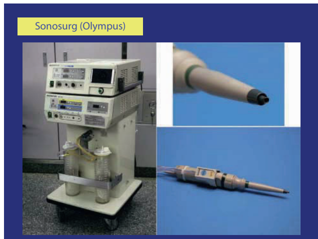
Fig. 49. Sono Surg (Olympus). By fitting an electric coagulation function to an ultrasonic histotripsy device, liver-cutting performance in cases of cirrhosis was improved
