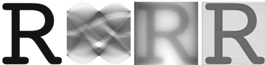
Figure 12.4.1 From left: letter R; its Radon transform (abscissa: angular variable); numerical inverse Radon transform; inverse Radon transform using a filter
