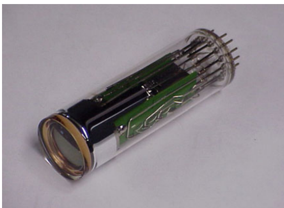
Fig. 5.2 An example of a photomultiplier tube (PMT)
