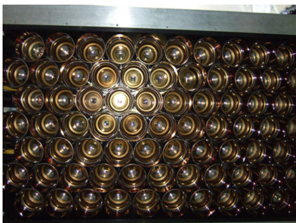
Fig. 5.26 CERN's LHCb-Rich detector using hybrid PMTs
