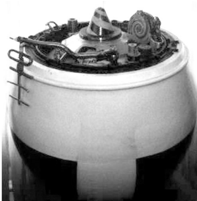
Figure 13.3 Venera 8 probe. Radio altimeter deployed at left, primary antenna in the center, secondary antenna and deployment mechanism at the right. Small cylinders on the rim are the two photometers, one on each side, and the gas analyzer.
