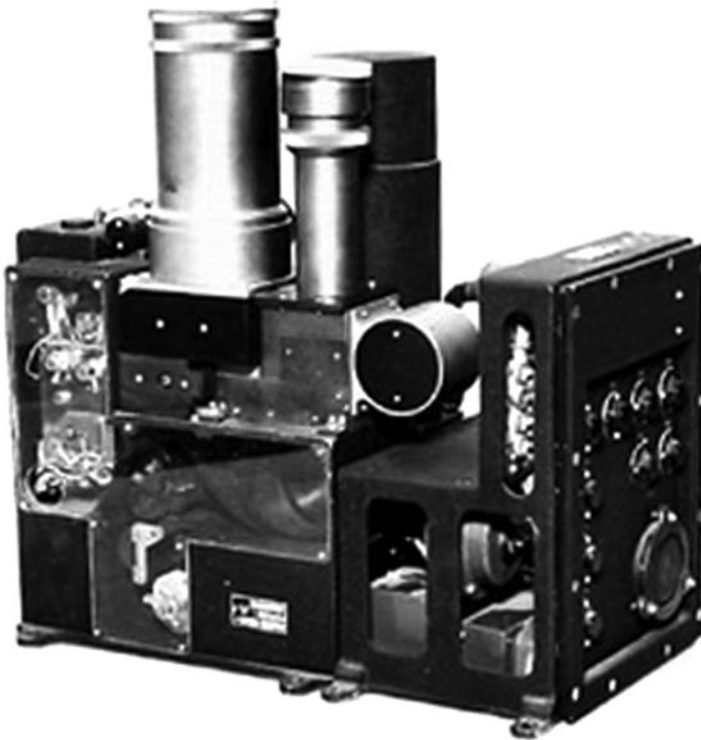
Figure 6.9 Yenisey-2 photo-facsimile imaging system.
