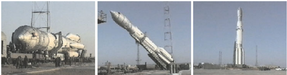
Figure 4.7 Transport and erection of the Mars-96 Proton-K vehicle.
