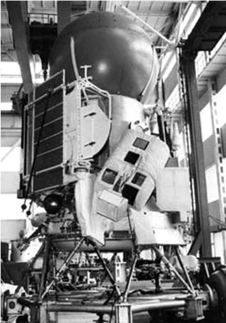
Figure 18.3 Vega 1 folded and ready to launch. Note scan platform, insulation and metal shielding.
