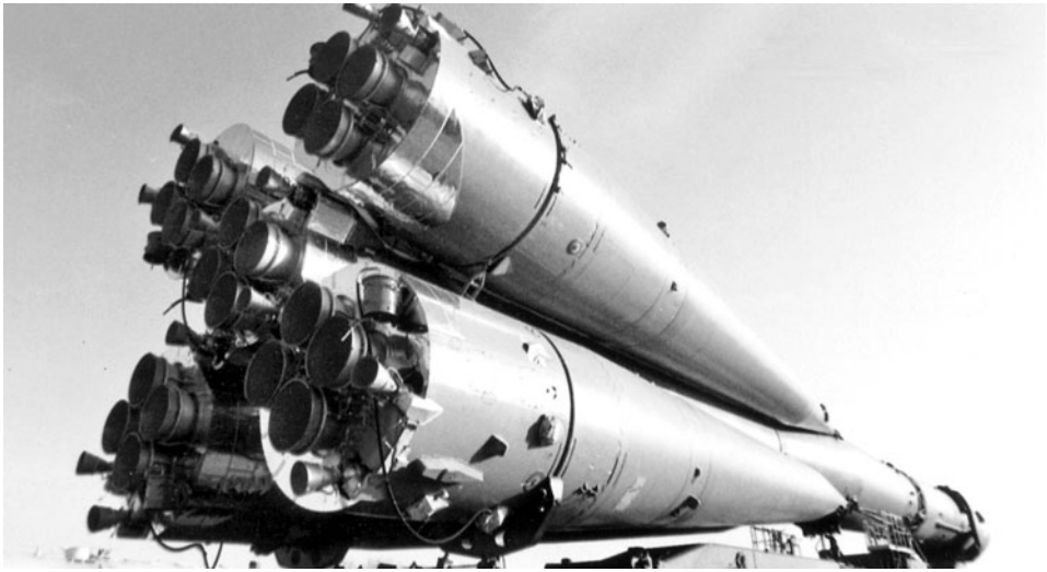
Figure 4.4 R-7 vehicle on rail carrier.
