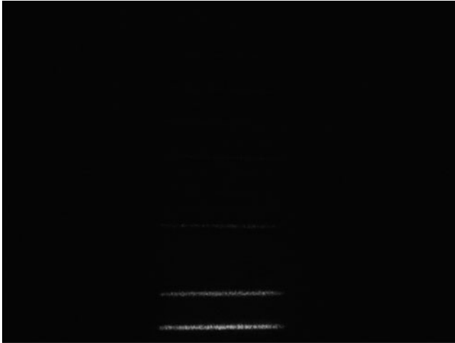
Fig. 3.20 Output of cosine setup with coherent illumination. The image was taken from: J. Solomon, Z. Zalevsky and D. Mendlovic, “Super Resolution Using Code Division Multiplexing,” Appl. Opt. , 42, 1451–1462 (2003)
