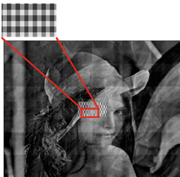
Fig. 2.8 The obtained result after the digital decoding. One may see the full field of view and the zoomed highly resolved barcode pattern in the center of the field of view. The image was taken from: Z. Zalevsky and A. Zlotnik, "Single Snap-Shot Double Field Optical Zoom," Opt. Exp. 13, 9858–9868 (2005)
