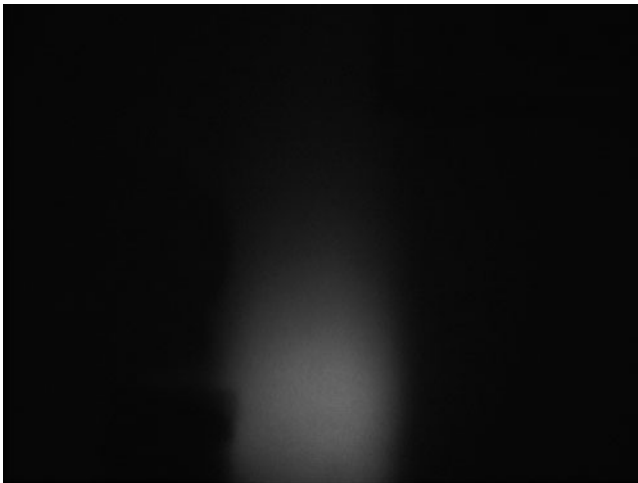
Fig. 3.21 Output of the cosine setup for incoherent illumination but without a mirror. The image was taken from: J. Solomon, Z. Zalevsky and D. Mendlovic, “Super Resolution Using Code Division Multiplexing,” Appl. Opt. , 42, 1451–1462 (2003)
