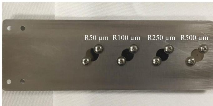
Fig. 4.25 The stainless-steel plate with tungsten collimators. The R50 \mu\text{m} collimator was not installed in the high power test
