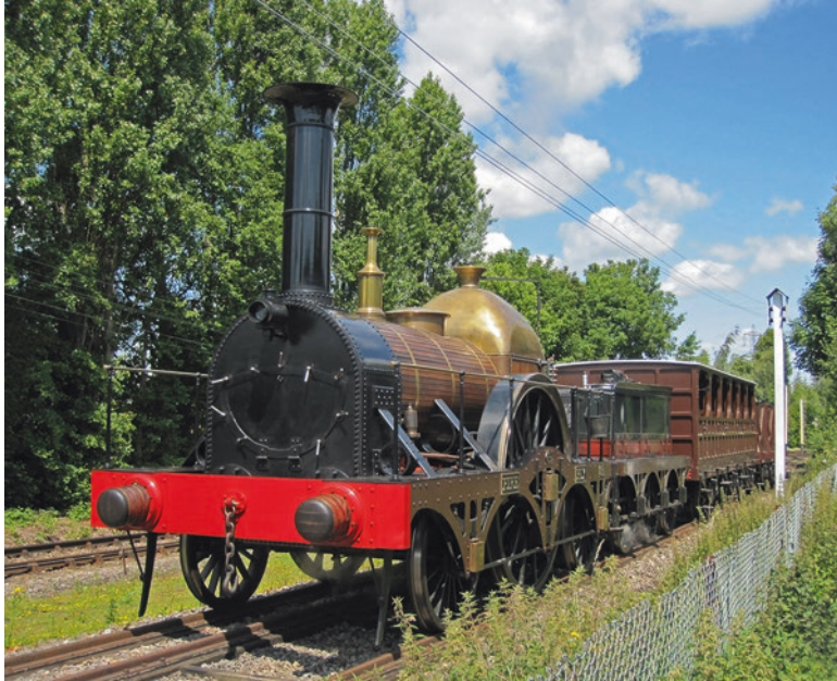
Fig. 10.3 The Fire Fly class of locomotives provided motive power for Great Western Railway passenger trains during the 1840s. This replica of the original Fire Fly was constructed in 2005 and is now displayed at the Didcot Railway Center, where it runs under steam on a special broad gauge line (Photograph by Peter Turvey. Used with permission)
