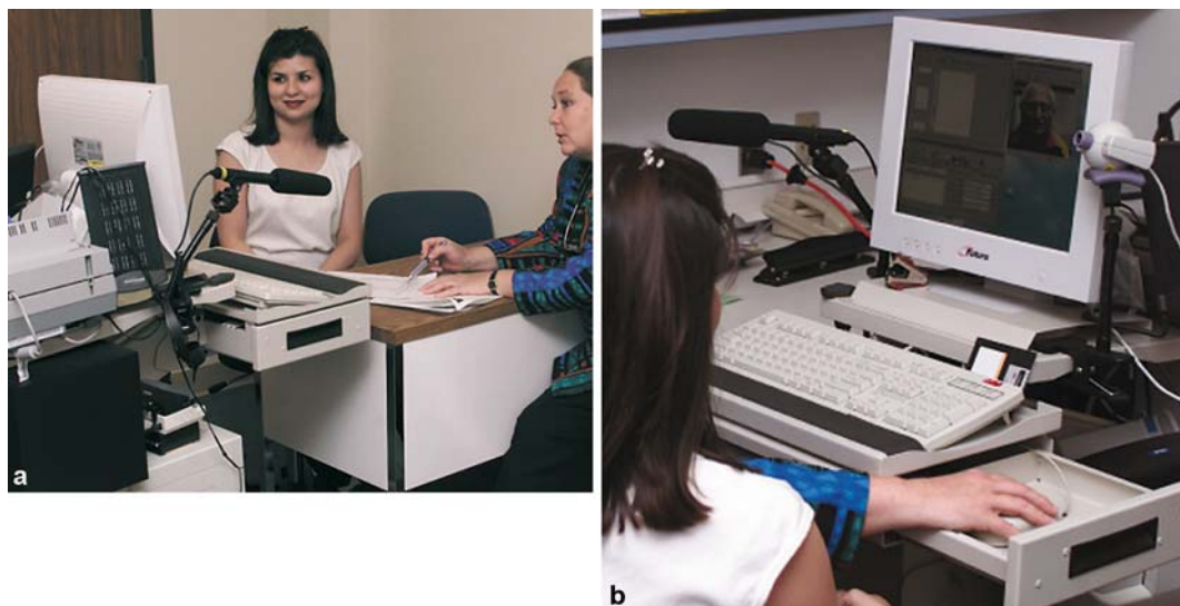
Fig. 15.1. a Telemedicine mobile cart with flat screen monitor ( left ). b Peripheral devices such as flat bed scanner with automatic document feeder, microphone, speakers, video camcorder with tripod, and projector ( right )
