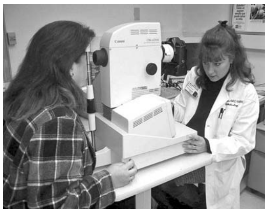
Fig. 13.1. Measuring device for optec visual acuity. This self-contained desktop unit incorporates its own illumination and optics. We use a log-mar test target based on the ETDRS target, providing measurements from 20/200 to 20/12. To overcome possible refractive errors, a pinhole attachment is inserted when the patient cannot read better than 20/50
