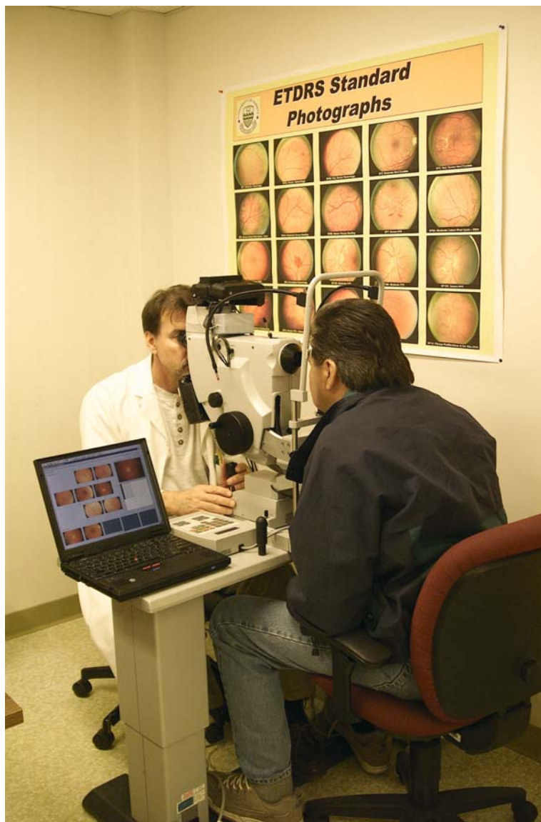
Fig. 16.2. University of Alberta Teleophthalmology Capture System (Zeiss FF450 retinal camera linked to Kodak DCS760 digital back)
