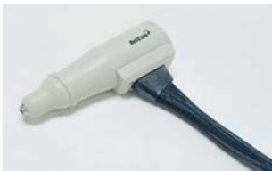
Fig. 14.1. Hand-held image capture unit for RetCam contains optics, focusing motor, megapixel CCD, and connecting cable to cart
