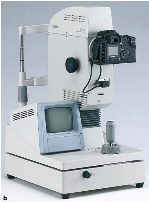
Fig. 2.12. Fundus cameras that are new, whether standard angiography models (a) or non-mydratic (b), are available with digital output. Some models were developed specifically for telemedicine applications. Images courtesy of Carl Zeiss Meditec, Dublin, California (a); Canon USA, Lake Success, New York (b); and Topcon America Corporation, Paramus, New Jersey (c)
