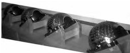
FIGURE 5.14 Four model U gamma knife radiosurgery collimator helmets produce 4, 8, 14, and 18mm beam sizes. They are changed manually between treatment shots as needed.
