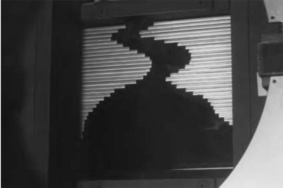
FIGURE 2.3 Typical multileaf collimator, used to shape the beam. Photo courtesy of Elekta.
