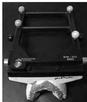
FIGURE 5.18 The dental mold and optical tracking system attachment is shown above. (Used with permission of Varian, Palo Alto, CA).
