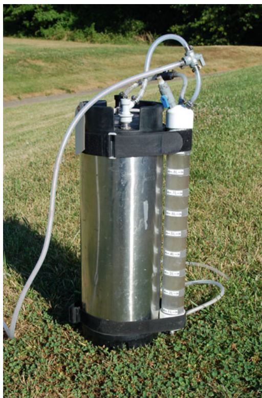
Figure 3.12. Stainless steel soda keg (5 gal/18.5 L) with attached measuring device, used to deliver and inject Dhc -containing cultures. Most bioaugmentation vendors now use these, or similar, containers to maintain anaerobic conditions during transport and injection of bioaugmentation cultures. The attached measuring device is calibrated to allow accurate delivery of a desired culture volume while maintaining anaerobic conditions.
