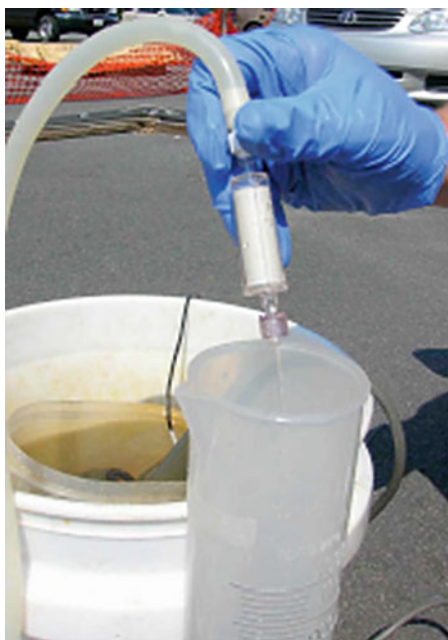
Figure 6.2. Sterivex™ filter used for groundwater sampling for MBT analysis (photo courtesy of MO BIO Laboratories, Carlsbad, CA).
