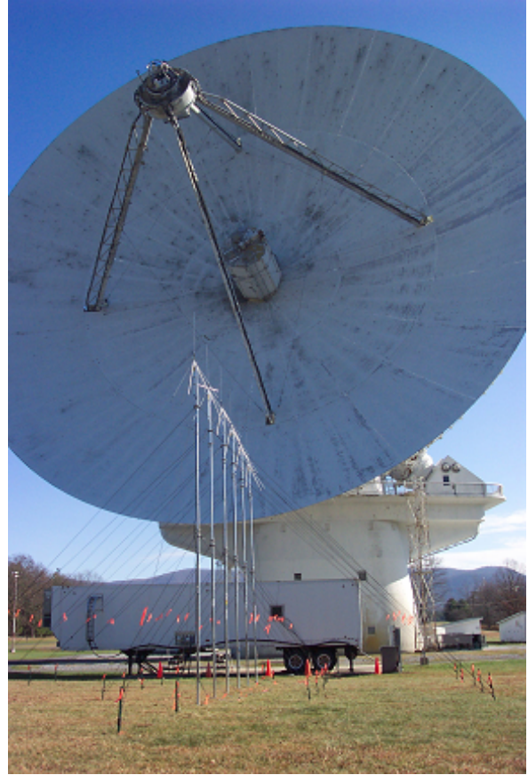
FIGURE 3.4 Left , an ISIS receiver deployed in the field at the National Radio Astronomy Observatory (NRAO) at Green Bank, W.Va. Courtesy of Massachusetts Institute of Technology. Right , foreground, is the Discone antenna array used by the ISIS node at Green Bank. In the background is the Green Bank 140-ft antenna. Courtesy of Glen Langston, NRAO. NRAO is a facility of the National Science Foundation operated under cooperative agreement by Associated Universities, Inc.
