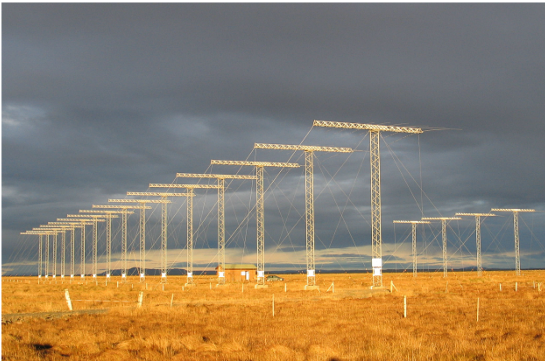
FIGURE 3.3 SuperDARN radar at Stokkseyri, Iceland. SOURCE: Courtesy of Jean-Paul Villain, French National Centre for Scientific Research.
