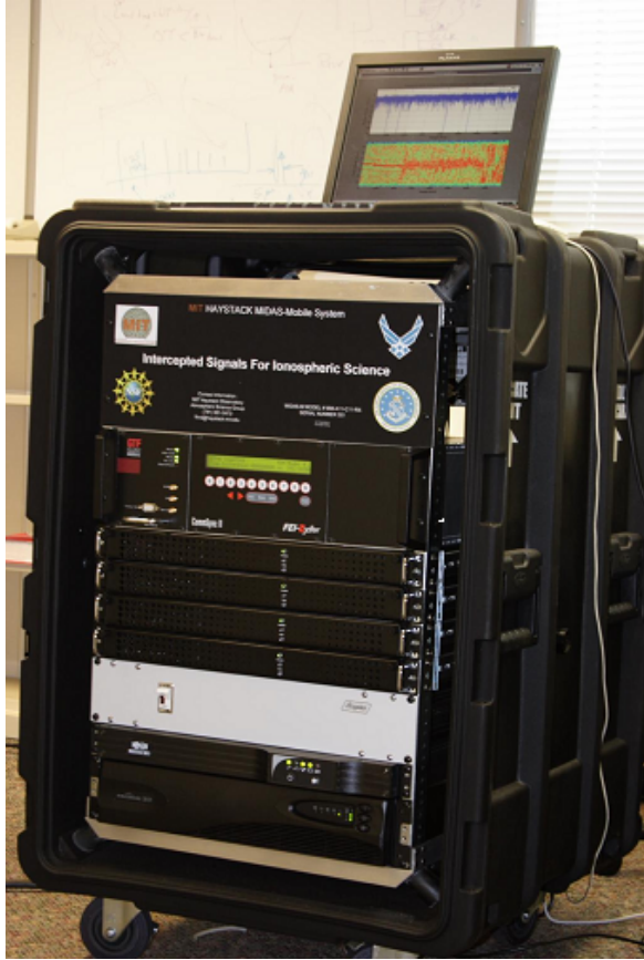
FIGURE 3.4 Left , an ISIS receiver deployed in the field at the National Radio Astronomy Observatory (NRAO) at Green Bank, W.Va. Courtesy of Massachusetts Institute of Technology. Right , foreground, is the Discone antenna array used by the ISIS node at Green Bank. In the background is the Green Bank 140-ft antenna. Courtesy of Glen Langston, NRAO. NRAO is a facility of the National Science Foundation operated under cooperative agreement by Associated Universities, Inc.
