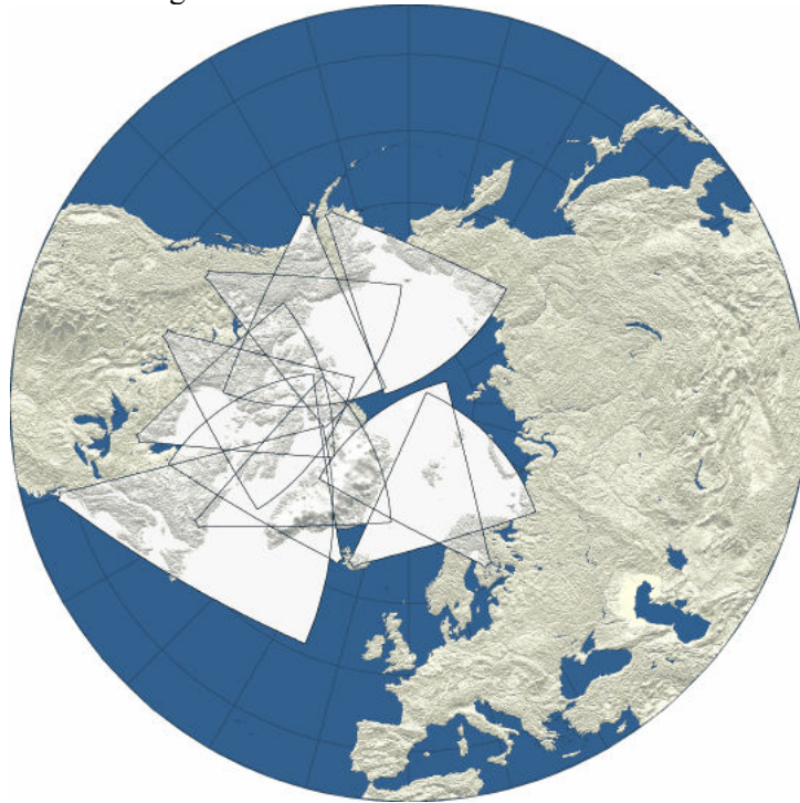
FIGURE 2.2.1 Graphic from the SuperDARN home page on the World Wide Web that shows the fields of view of the northern SuperDARN radars. SuperDARN sites are also present in the Southern Hemisphere. See superdarn.jhuapl.edu/ . SOURCE: Johns Hopkins University Applied Physics Laboratory.
