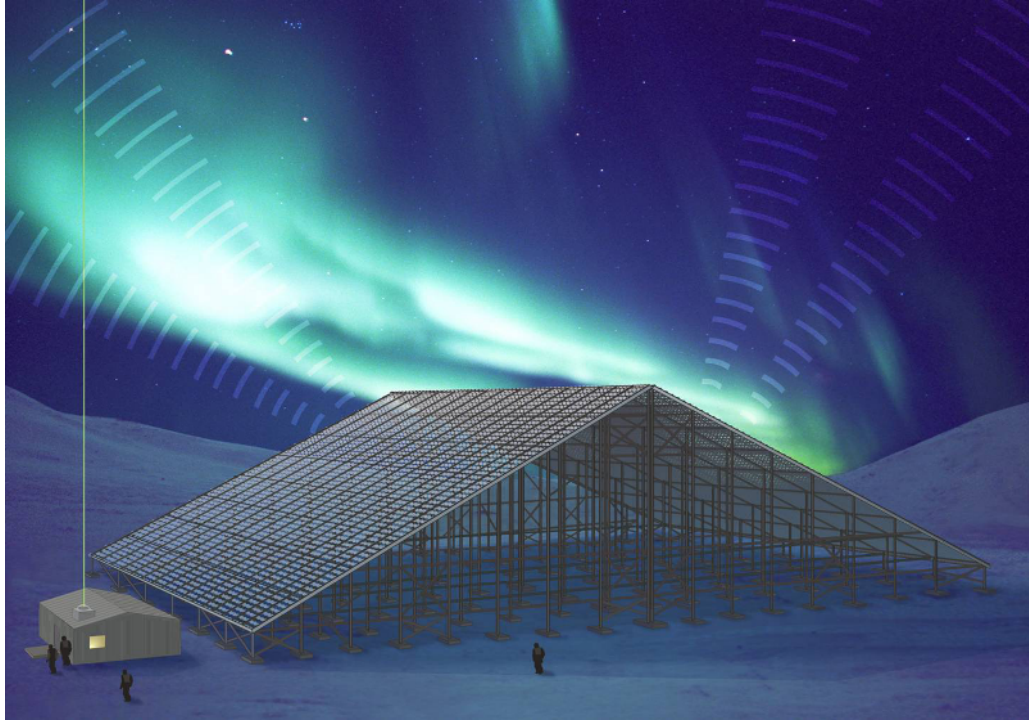
FIGURE 3.2 Artist's concept of the portable Advanced Modular Incoherent Scatter Radar deployed at a high-latitude site to study the response of the upper atmosphere to auroral activity. SOURCE: Courtesy of J. Kelly and C.J. Heinselmann, SRI International.
