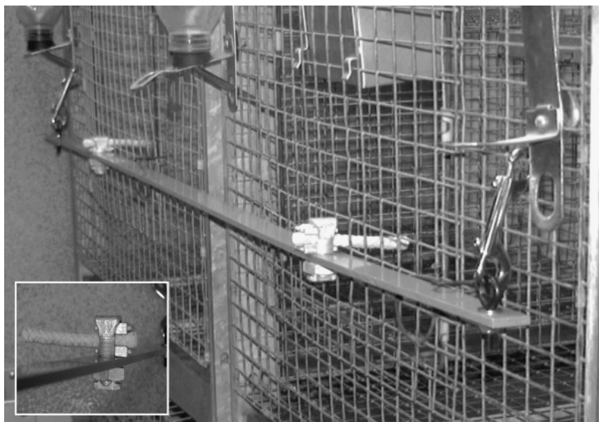
Figure 21-2. Fully assembled SPIT, mounted and ready for sampling. Inset: closeup of the split-bolt assembly with SPIT Stick.
