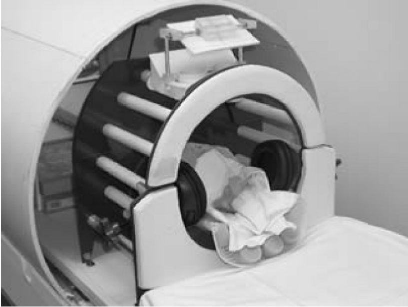
Figure 23–6. Photograph of volumetric head coil. The subject's head is positioned inside the coil.
