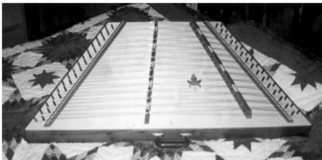
Fig. 21.1 A basic hammered dulcimer with 15 treble courses and 15 bass courses with birch soundboard and walnut rails, made by author
