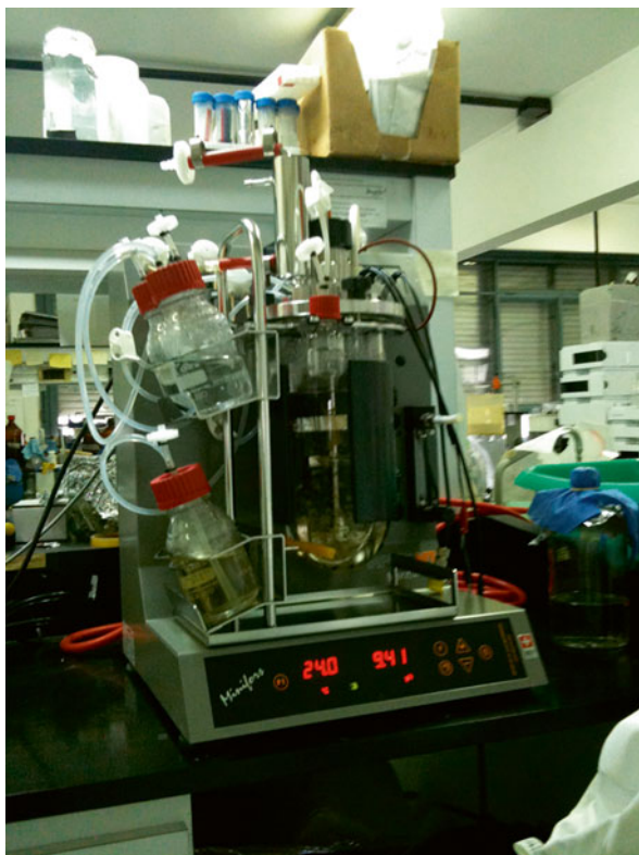
Fig. 7.14 2-l bioreactor inoculated with MSRT culture media without plant growth regulators for growing N. tabacum cell suspension culture line Ab-KDEL
