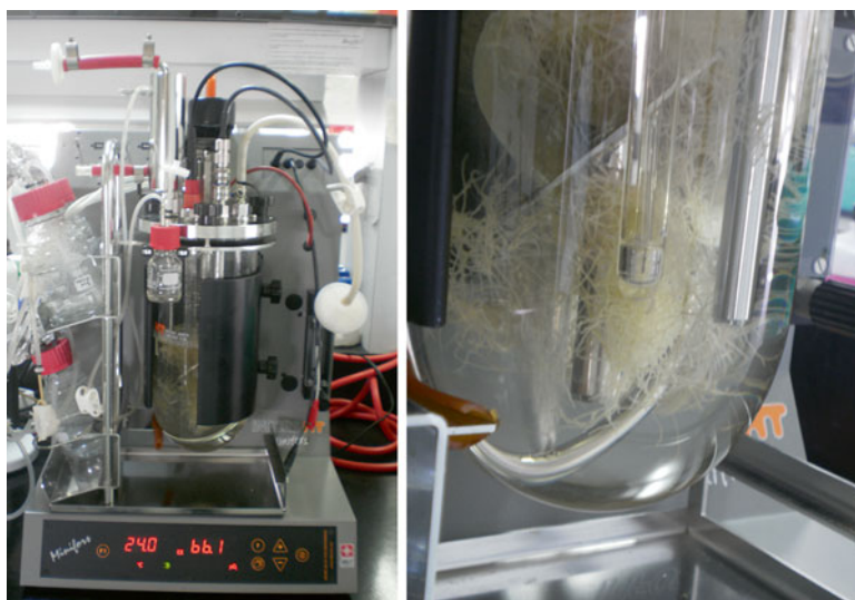
Fig. 7.8 N. tabacum hairy roots, line sec-Ab growing in a 2 l- bioreactor (Minifors) in MSRT media without plant growth regulators
