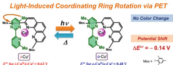
Fig. 4.1 Conceptual diagram showing the photo- and heat-driven pyrimidine ring rotational isomerization of 3\cdot\text{BF}_4
