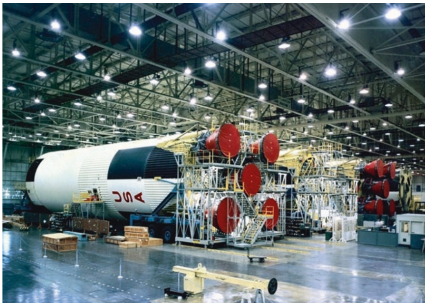
Fig. 5.6 Engines being installed on S-1C stages at Michoud (NASA photo)
