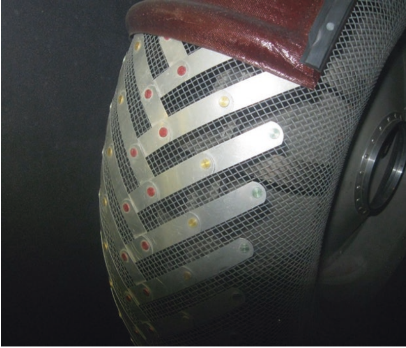
Fig. 10.3 Wheel of LRV showing wire mesh construction and titanium chevron tread (NASA Photograph)
