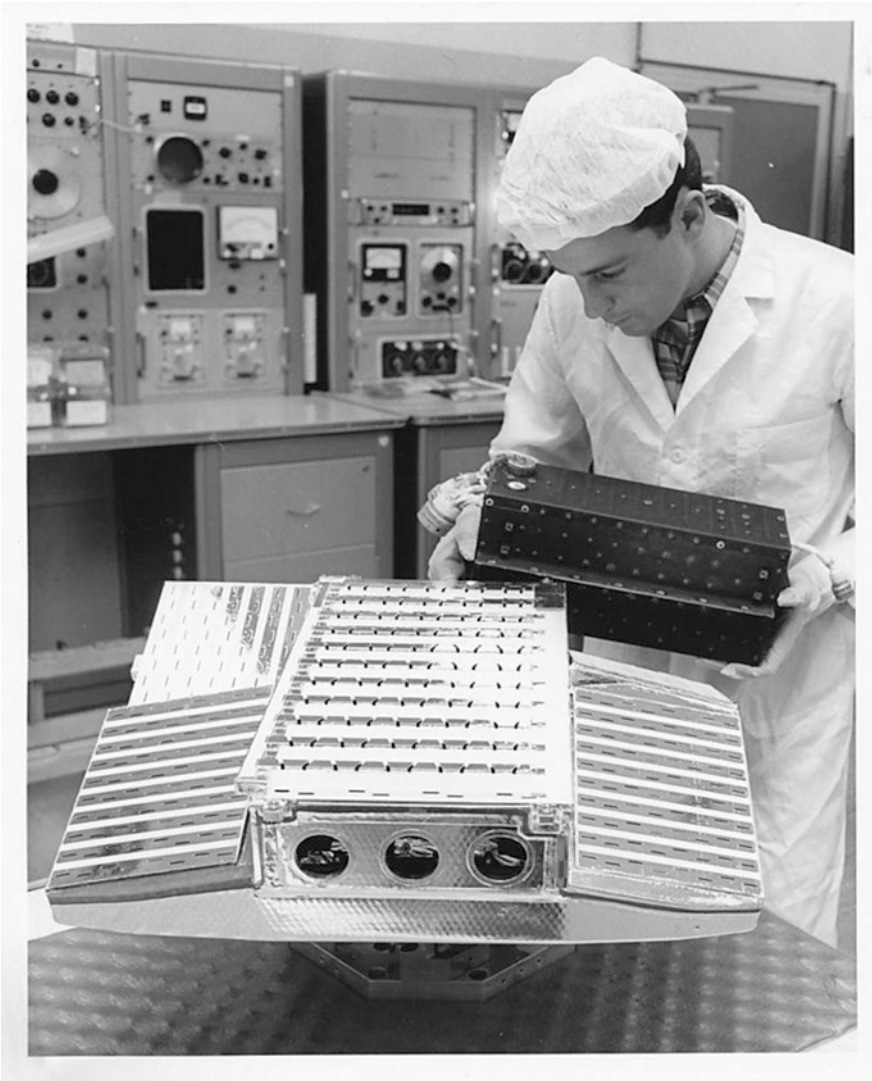
Fig. 8.19 Antenna assembly of landing radar resting on a bench and electronics assembly being carried (from author's files)
