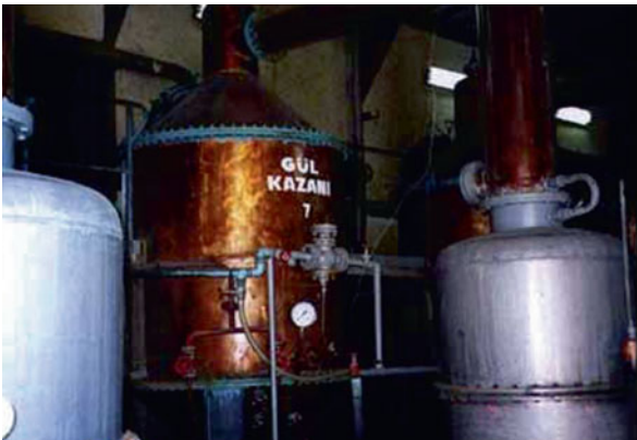
3.10 Production of rose oil by steam distillation in Turkey.
