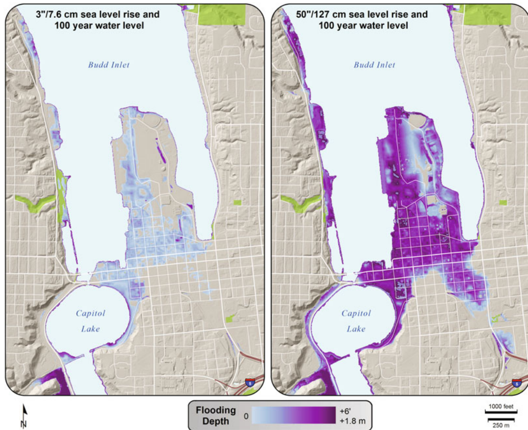
Figure 4.6 Projected flooding of downtown Olympia with a 100-year water level and 127 cm (50 in) of sea level rise. Redrawn from Coast and Harbor Engineering (2011).
