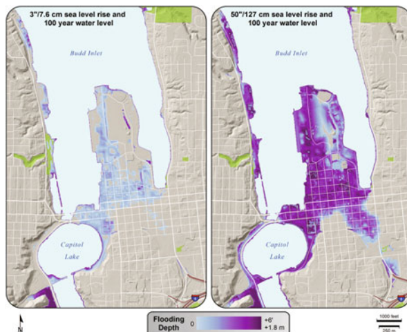
Figure 4.6 Projected flooding of downtown Olympia with a 100-year water level (0.01 average annual exceedance probability for storm tides, wave effects on mean water level at the shoreline, and precipitation run-off) and 7.6 cm (3 in) of sea level rise (left) and a 100-year water level and 127 cm (50 in) of sea level rise (right). Redrawn from Coast and Harbor Engineering (2011), courtesy City of Olympia.
