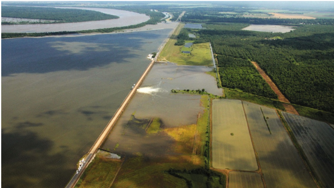
On May 14, 2011, the US Army Corps of Engineers opened the first gate on the Morganza Floodway in Louisiana to relieve flooding on the Mississippi River. Source: US Army Corps of Engineers; http://www.flickr.com/photos/30539067@N04/5722952407 .
