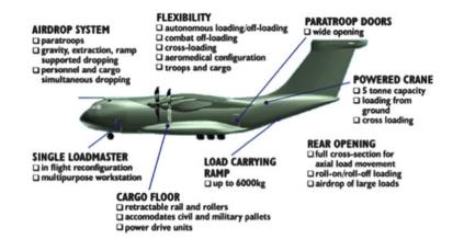
**Fig. 12.32** The main characteristics of the A400M (Picture from the Airbus Military Company website: airbusmilitary.com)
