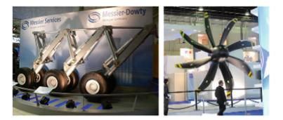
**Fig. 12.34** A400M landing gear (by Messier Dowty) displayed at Paris Air Show in 2007, and the A400M propeller (Hamilton Sundstrand) at the Paris Air Show in 2009 (Picture from the Airbus Military Company website: airbusmilitary.com)
