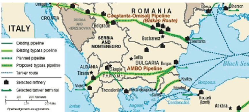
Figure 3. Balkan oil transit pipelines projects.
