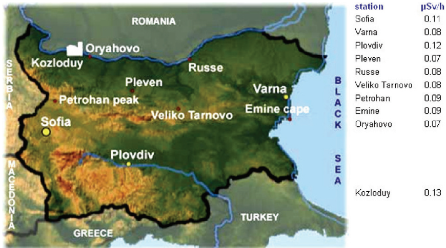
Figure 6. Average values of current radiation gamma-background in Bulgaria for the last 24h at 09:00 on 18 October 2007. For the territory of the Republic of Bulgaria the natural gamma-background is from 0.06 to 0.60 \mu\text{Sv/h} .
