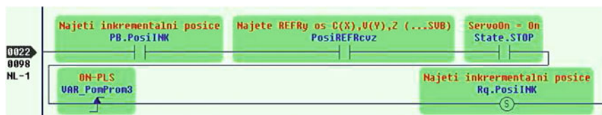
Fig. 3 Definition of input variable [B]On/Off of the POSI-INK function
