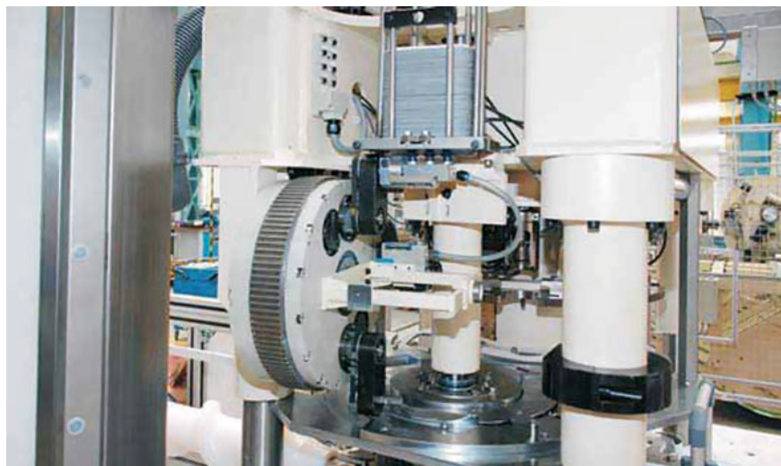
Fig. 4 Arrangement of the separating mechanism
