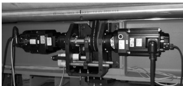
Fig. 4 New conception of the main drive using Yaskawa servomotors
