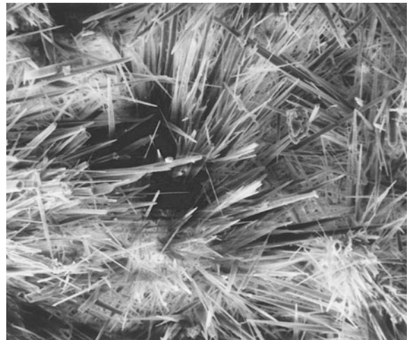
Fig. 23.21 Scanning electron microscope image of the tip of an aragonite needle. Magnification 2675X
