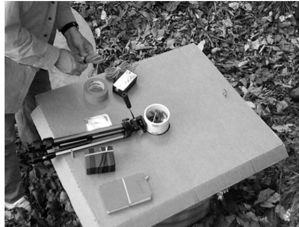
Fig. 22.15 Cardboard has been placed over the entrance (a vertical culvert pipe) to Basswood Cave. The anemometer placed over a hole in the cardboard records the rate of air flow (photo by P. C. Lucas)
