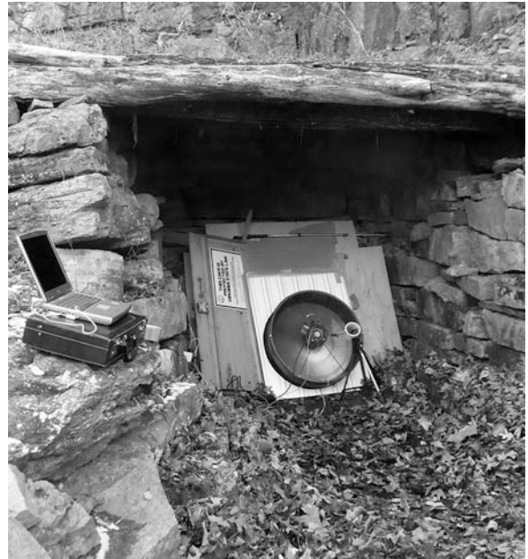
Fig. 22.11 The rectangular doorway Butler Cave's SOFA entrance has been sealed around a fan. The fan blows alternately in and out of the cave in even intervals. A signal is sent from the fan to a recording data logger when the fan changes direction (photo by P. C. Lucas)
