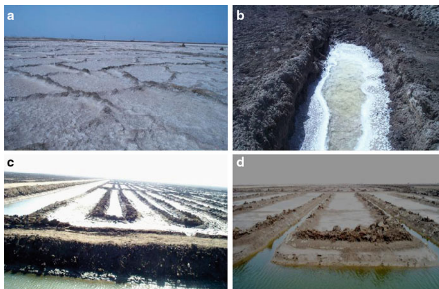
Fig. 48.2 Experimental area, surface salt crust (a), shallow groundwater table (b), leaching process (c) and after removing surface salt crust (d)
