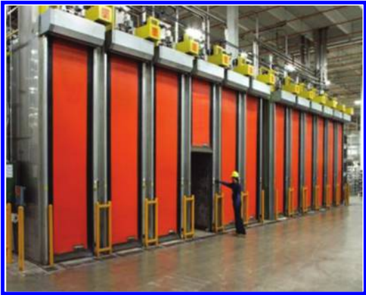
FIGURE 7.19 Curing chamber. (From International Thermal Systems. Available at http://internationalthermalsystems.com/batterymanufacturing. )
