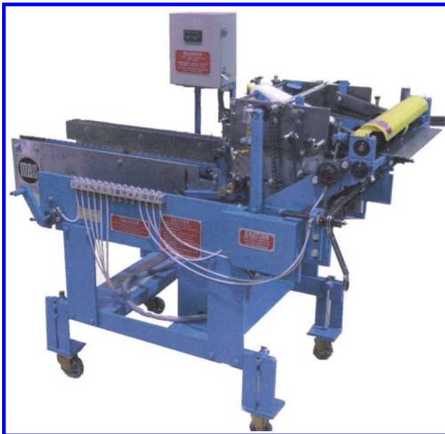
FIGURE 7.15 Grid feeder. (From MAC Engineering. Available at http://www.mac-eng.com .)
