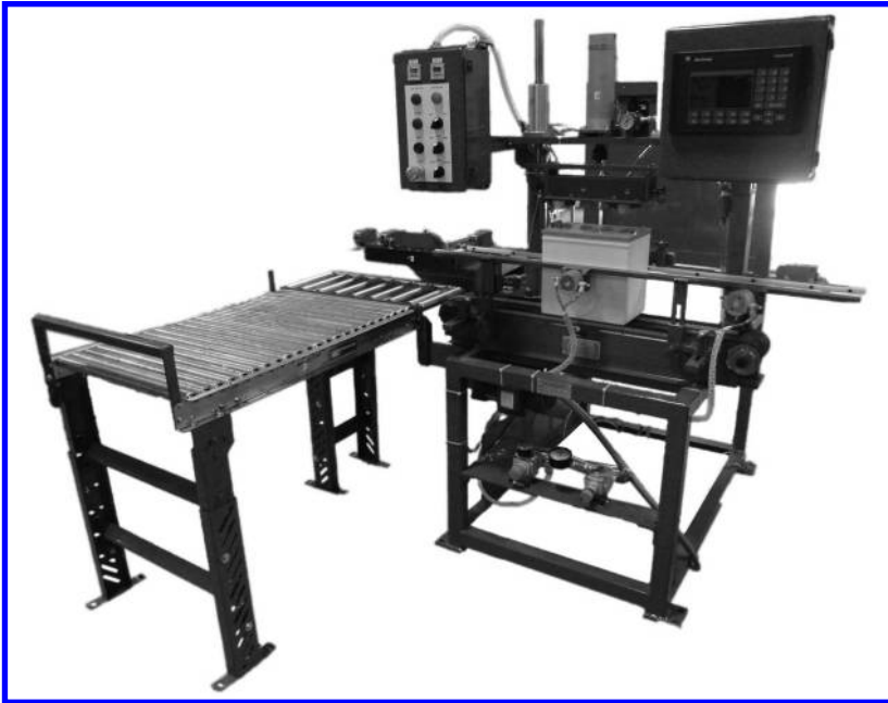
FIGURE 7.29 Leak testing machine. (From MAC Engineering. Available at http://www.mac-eng.com .)
