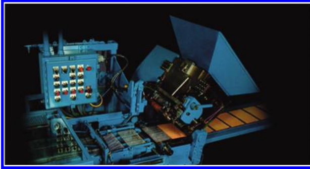
FIGURE 7.14 Continuous orifice paster. (From Wirtz Manufacturing. Available at http://www.wirtzusa.com .)
