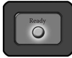
FIGURE 8.1 The “ready” light lies. The READY light indicates that the battery is fully charged. This does not mean “able.” There is no link between “ready” and battery performance.
