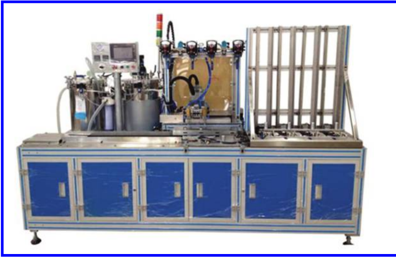
FIGURE 7.28 Epoxy sealing system.
