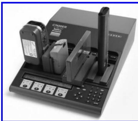
FIGURE 8.5 Cadex C7400ER battery analyzer. Two- and four-station analyzers service batteries from 1.2 to 36 V, using unique algorithms for lead, nickel, and lithium-based chemistries. (Courtesy of Cadex.)
