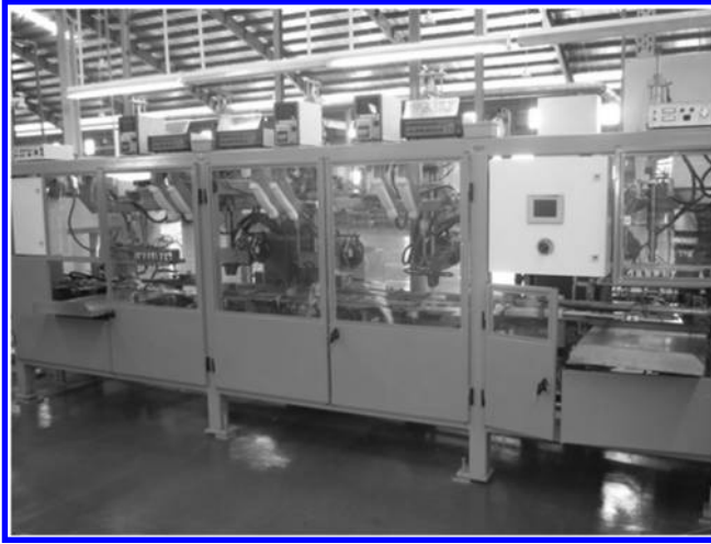
FIGURE 7.26 Intercell welding machine. (From Wirtz Manufacturing. Available at http://www.wirtzusa.com .)
