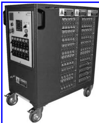
FIGURE 8.4 Load banks to discharge large battery systems for a performance check. The capacity of critical standby batteries is often measured by applying a full discharge. Such a test can take more than a day to perform.
