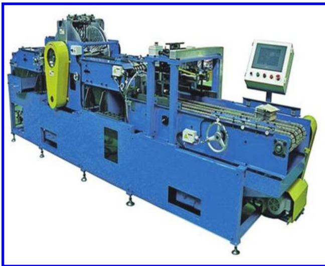
FIGURE 7.18 Stacker. (From International Thermal Systems. Available at http://internationalthermalsystems.com/batterymanufacturing .)
