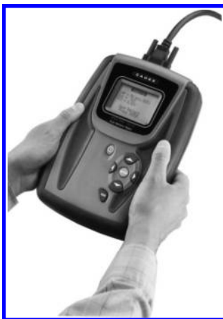
FIGURE 8.13 The Spectro CA-12 compact battery rapid tester displays capacity, CCA, and SOC in 15 sec. Capacity reflects the true state of health of a battery.
