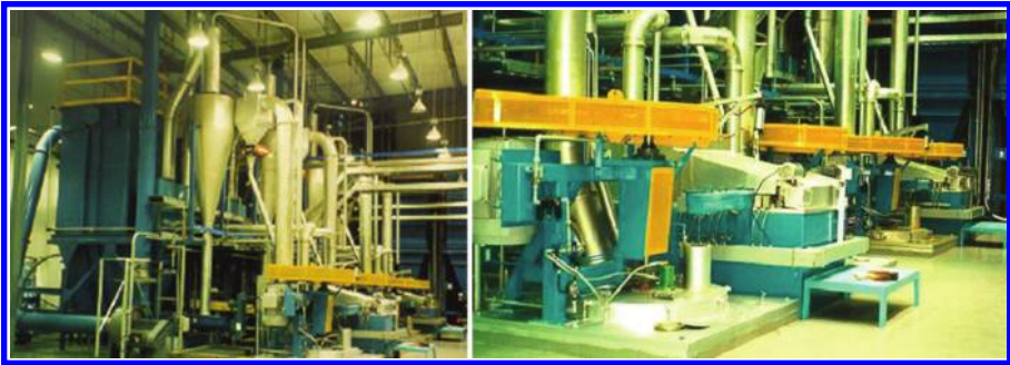
FIGURE 7.8 Barton pot. (From Wirtz Manufacturing. Available at http://www.wirtzusa.com .)
