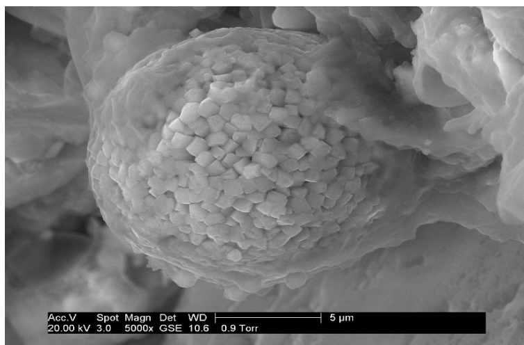
Figure 2. Iron sulfide framboid from black layer formed in a sand-based turfgrass rootzone.
