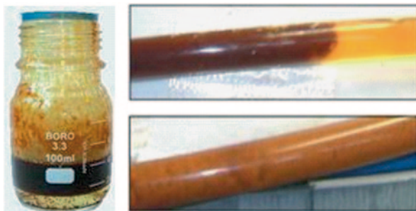
Fig. 1.5 Extremely concentrated solutions ( left ) can be injected in a CCC column. The right part of the figure shows a partial precipitation that occurred inside the injection loop during large scale natural product extract purification. The chromatogram developed normally. Adapted from (Freebairn et al. 2011) and Dynamic Extractions with permission
