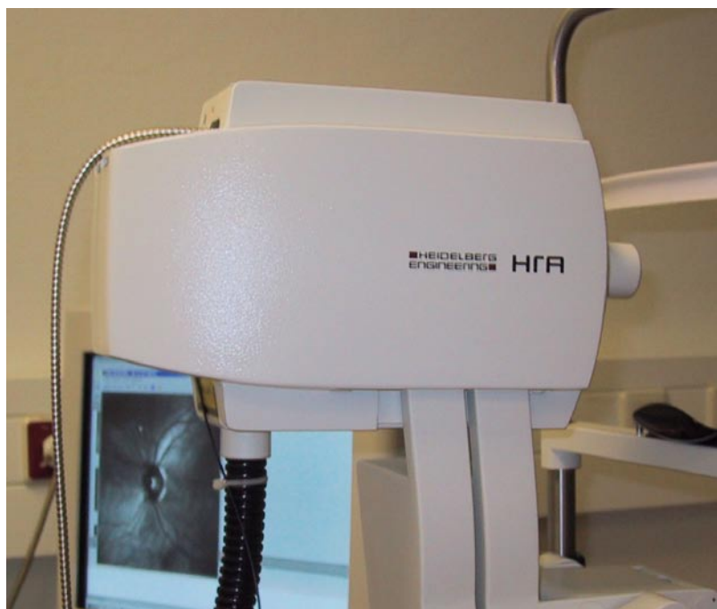
Fig. 6.1 Modified confocal scanning laser ophthalmoscope for macular pigment measurement
