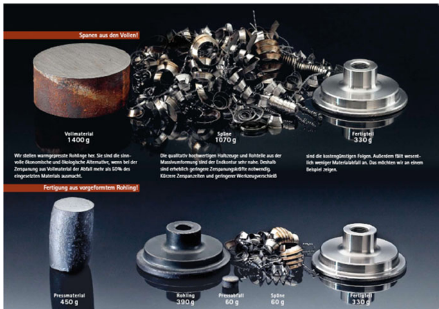
Fig. 9.4 Using preformed blanks instead of solid material
