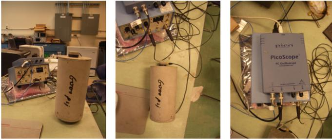
FIG. 4. Ultrasonic testing device and example photos of testing concrete specimen
