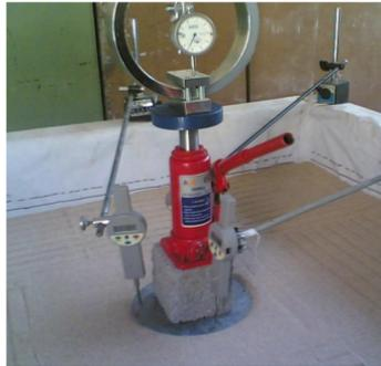
**FIG. 2. The arrangements of jack and gauges on the foundation.**
