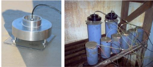
FIG. 3. a) TDR sensor head with cable b) TDR sensor and thermocouple distribution
