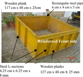
**FIG. 3. Panoramic view of Upper Shear Box.**
