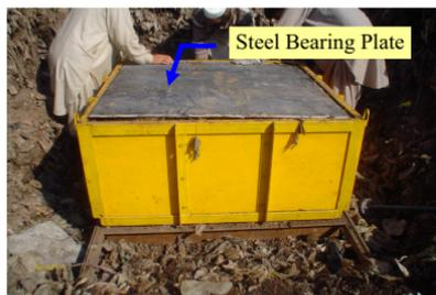
**FIG. 12.** Normal Load Bearing Plate placed over the specimen.
