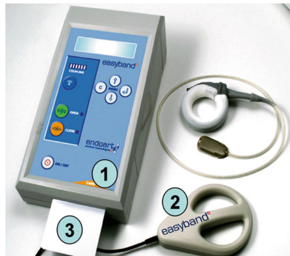
Fig. 2.5 Remote adjustable Gastric band (courtesy of Allergan). (1) A control unit sends energy and information telemetrically to the easyband through magnetic induction. (2) Antenna: magnetic induction is sent to the antenna, which is connected to the easyband. (3) A microchip saves the adjustments of the easyband
