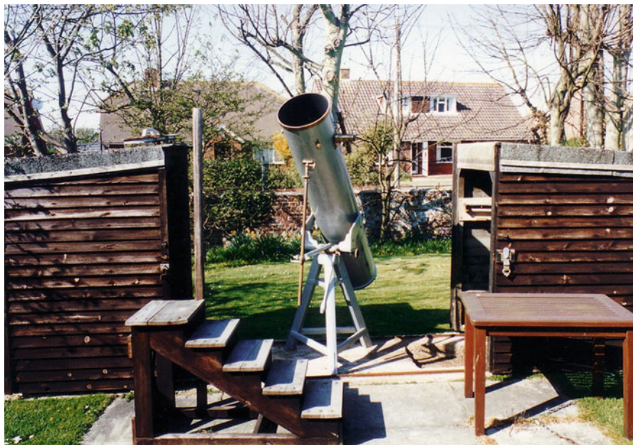
Fig. 9.2 Patrick's home-built 12½-inch Newtonian has a double run-off protective building
