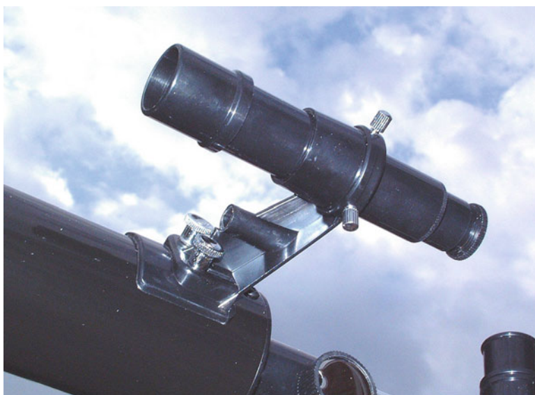
Fig. 2.5 A typical finderscope. Note the three adjustment screws
