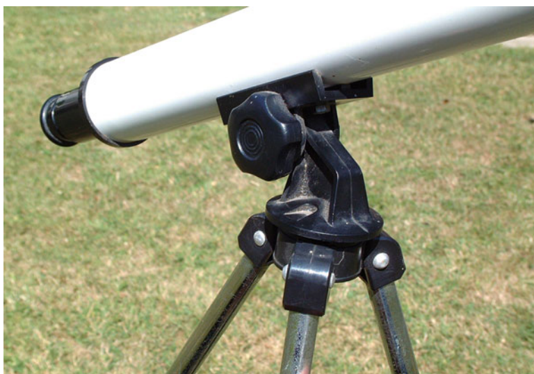
Fig. 1.3 An inadequate tripod
