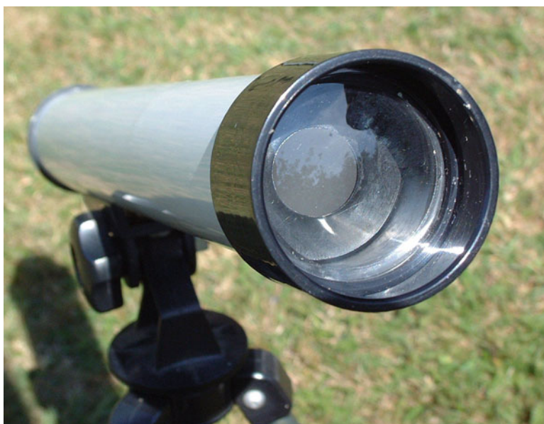
Fig. 1.2 Not quite what it seems – a small refractor fitted with an aperture stop
