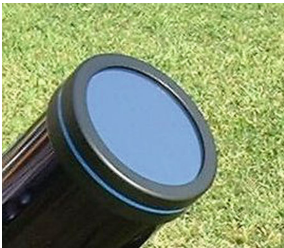
Fig. 4.9 A full-aperture solar filter – the only safe way to observe the Sun with an astronomical telescope
