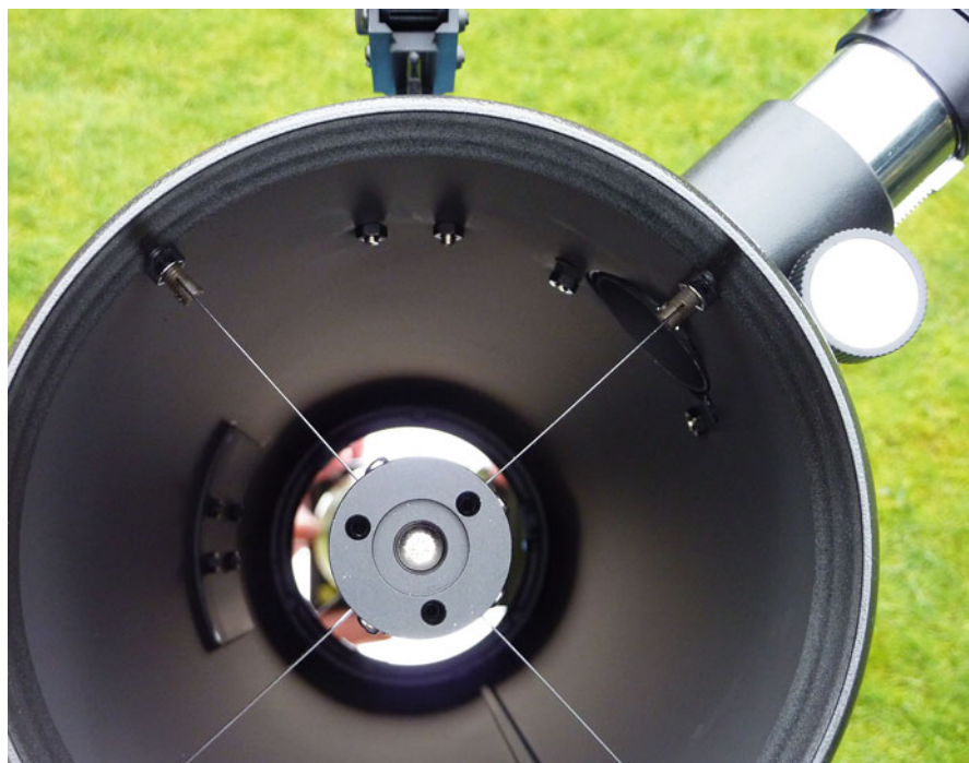
Fig. 8.10 The Sky-watcher secondary mirror is supported by four very thin tensioned steel vanes
