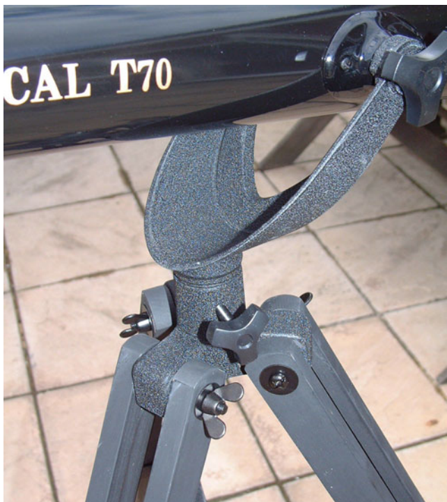
Fig. 2.8 A typical altazimuth mounting for a budget telescope
