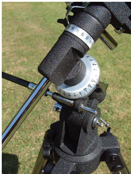
Fig. 2.9 A typical equatorial mounting for a budget telescope. Note the setting circles and the slow-motion cable for R.A. The declination cable is not fitted in this picture
