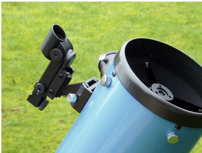
Fig. 2.6 A red dot finder, fitted to a 5-inch reflector
