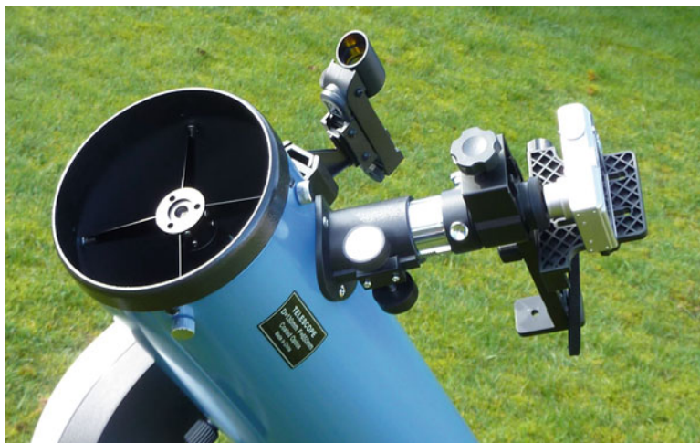
Fig. 6.3 An excellent purpose-made camera-bracket, the oddly named ‘Universal Digiscoping’
