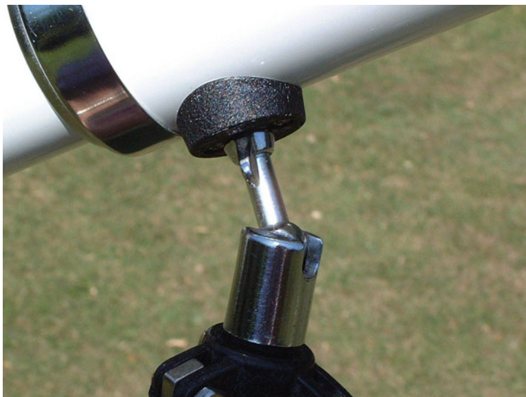
Fig. 2.7 Ball-and-socket – the very worst mounting for an astronomical telescope!
