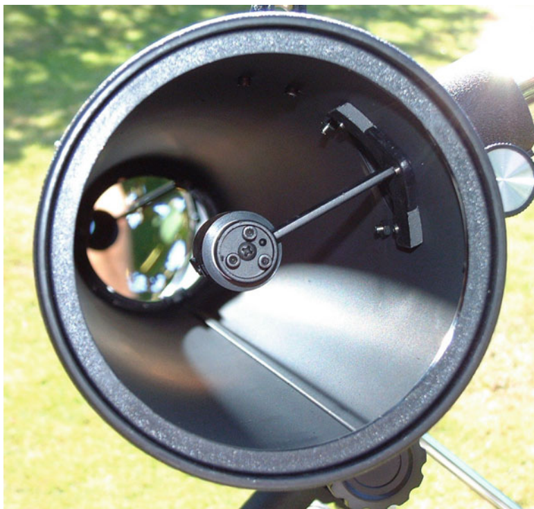
Fig. 8.3 The Luminova secondary mirror is supported by a single stout strut
