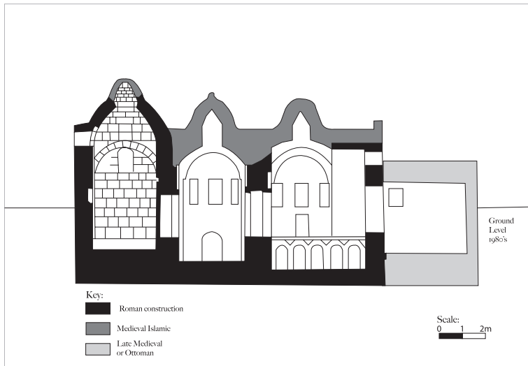
Fig. 6.4 Section through the shrine of Abu Ubayda at Emmaus showing different stages of construction (Drawing by Ifan Edwards)
