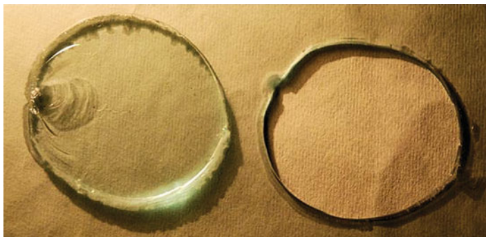
Fig. 1.6 A hole in the glass made by BL [21]. To the right, there is a hole in the glass; to the left, there is the disc that had fallen out the hole. Disc (hole) axes sizes are 8.2 and 7.6 cm, respectively
