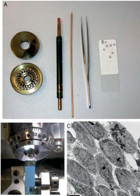
Fig. 6 (A) Tools required for cryosectioning from left to right A cryotransfer holder for carrying section covered grids between the cryoultramicrotome and freeze-drier, a copper rod used for pressing the sections onto the grids, an eyelash for picking up sections from the knife edge and transferring them to the grids, antimagnetic tweezers for handling Ni grids and Pioloform-covered Ni grids. (B) Interior of cryosectioning chamber ( -130^{\circ}\text{C} ) showing, the blockface a knife with a grid containing sections, the grid is supported on the knife by a tape strip. Sections are from the knife to the grid using an eyelash. (C) Freeze-dried cryosections of human neutrophils. The sections are compressed in the direction of cutting (arrow). The sections show high contrast despite the lack of staining, the contrast is due to differences in dry mass between the different organelles.
