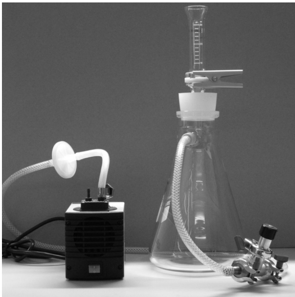
Fig. 2 Filtration system for sample harvesting (manual air inlet valve on the right).
