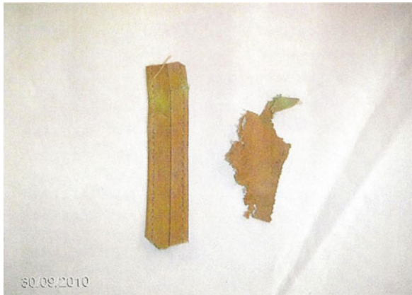
Fig. 16 Sample of unusable vinyl from Cantagalo Waste Separation and Composting Center
