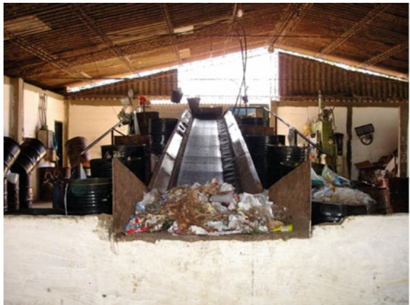
Fig. 2 Entrance of waste on the sorting conveyor belt
