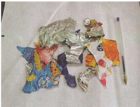
Fig. 11 Sample of aluminum foil from Cantagalo Waste Separation and Composting Center
